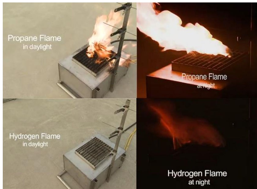
Figure 8.3. Propane Flame vs Hydrogen Flame (AIChE Academy, 2020)
